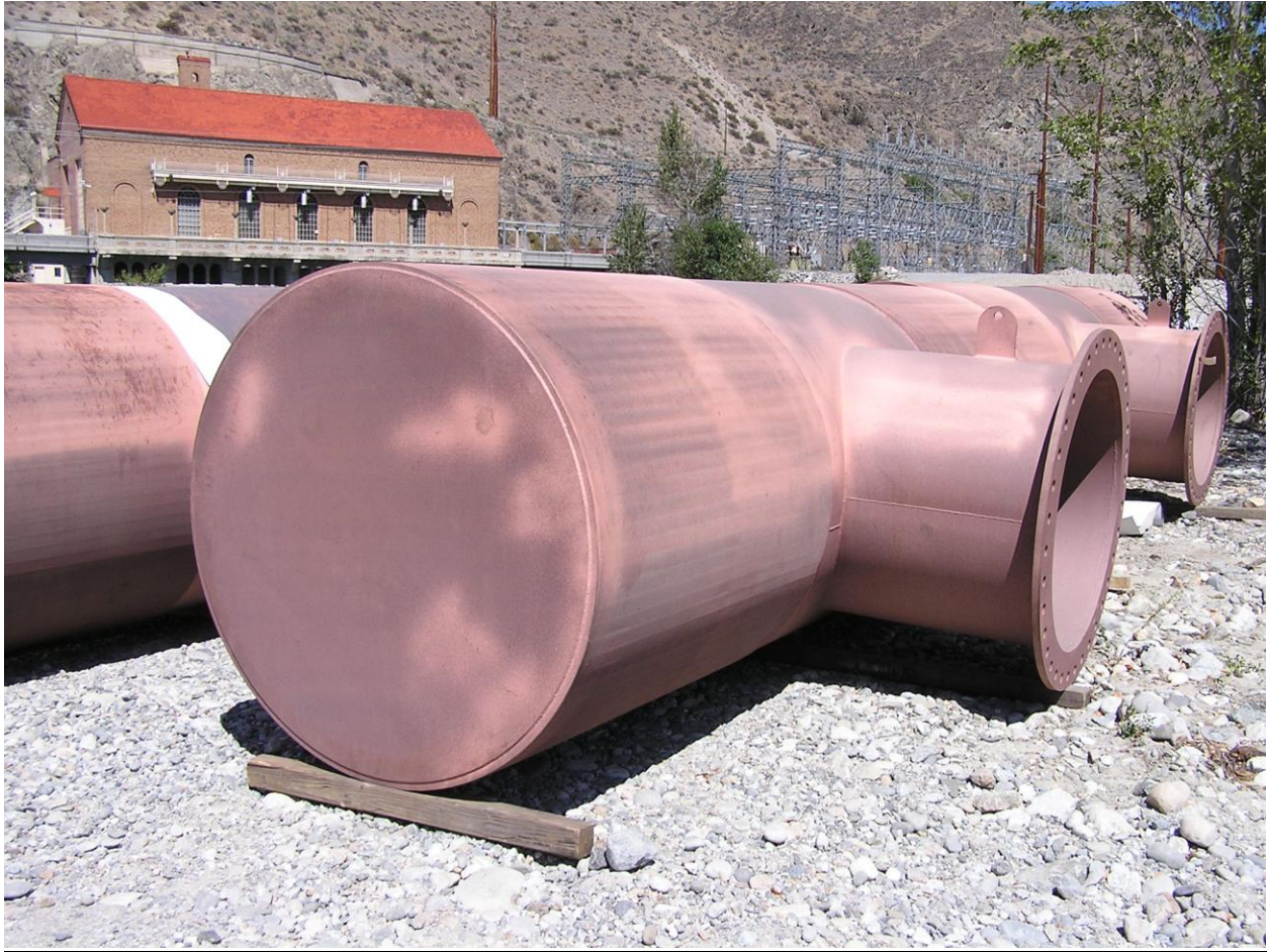
T-screens for the pump station intakes. August 12, 2008.
